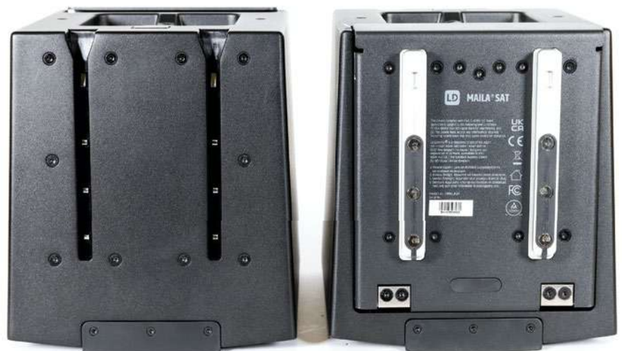
Connection of the satellites via rails with recessed contacts
