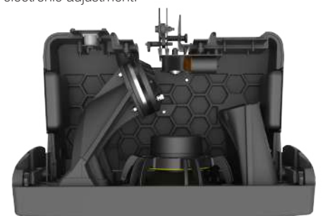
Internal view of the GEO M10 module, showing from left to right the HRW™ waveguide, the Neodymium 10" with PDD™ device and the curved V-shaped port.
