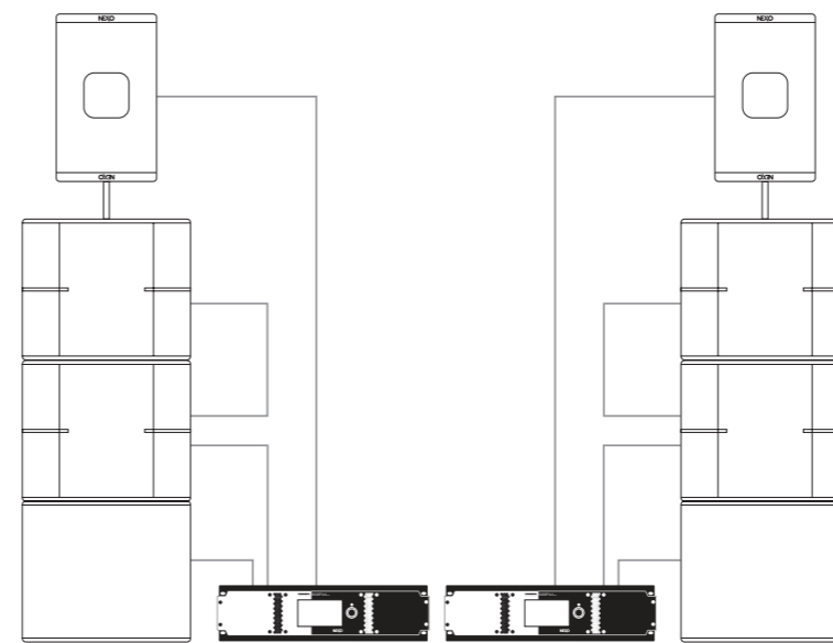
FOH System: (Per side) 1 x P18 (Passive) on 2 x L20 Subs on 1 x L20 Sub (Cardioid Mode), powered by 2 x NXAMP4X4MK2
