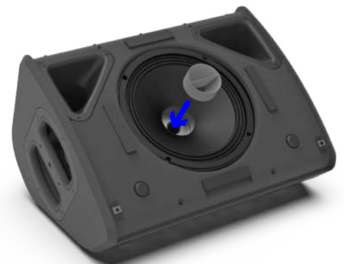
Grille removed, an optional magnetic horn can be quickly fitted to change directivity from 100°x100° to 110°x60°
