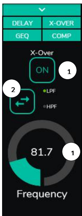
Figure 38: setting a crossover filter
